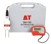
The kit comprises an SM150T Soil Moisture Sensor, a dedicated readout meter and a carry case. The cable and connector are watertight - an essential requirement for potentially wet environments.
